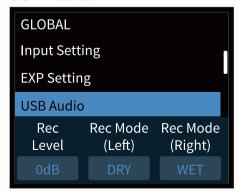
Use this menu to set up USB audio settings when using GP-100 as a USB audio interface. The Rec Mode options allow you to select USB recording input sources on left (L) and right (R) input channels. The selections for these are the same: dry signal (Dry) and wet signal (Effect). When recording, adjust the optimal Rec Level according to the instrument or other devices you're using.
