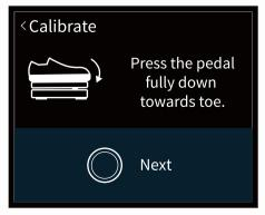
Then press the pedal all the way down (forward) and press the PARA button to select Next.
