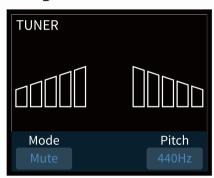
Press and hold both footswitches at any time to enter the tuner mode.
