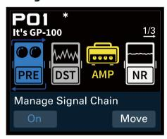
Press and hold the PARA button in the EDIT Menu to change the position of the effect module.
