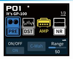
Turn the PARA knob or tap the footswitch to switch the patch. Press the PARA button or EDIT button to enter the EDIT menu. This menu is made of ten icon squares representing GP-100's nine effects modules.
