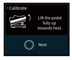
Bring the pedal all the way up (back) and press the PARA button to select Next.
