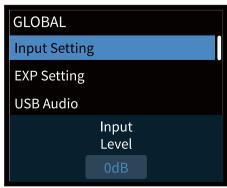
Set the global input levels and modes in the Input Settings menu. Adjust the optimal Input Level for the instrument or other sound source you're using. Adjustable range is from -20dB to +20dB. Default is set to 0dB.
