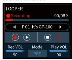
In the play mode, simultaneously press the [+]/[-] footswitches until the LOOPER menu appears.
