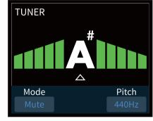
Quick access knob 3 adjusts the pitch calibration (REF PITCH), ranging from 435Hz to 445Hz. Standard pitch is set at 440Hz. Quick access knob 1 lets you select the tuner mode from Bypass (for dry signal through), Thru (for effect signal through) or Mute (for silent tuning). You can exit the tuner either by pressing any footswitch or by pressing the EXIT button.
